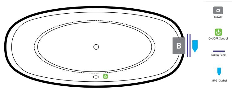
Airbath System II Factory installed blower may only be placed in this location.
