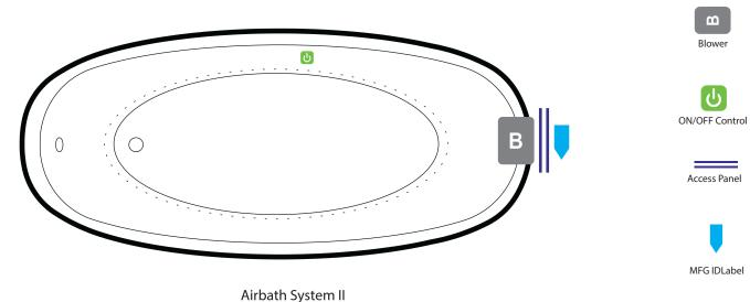
Factory installed blower may only be placed in this location.
