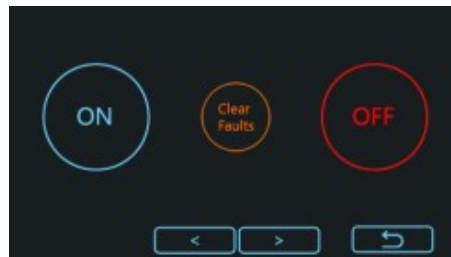
Fig. 5-11 Startup and shutdown control
