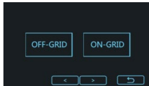
Fig. 5-12 Grid-tied and off-grid setting
