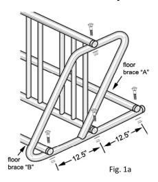
Step 1: Starting with one side, align the bike grid to the side rail as shown in Fig. 1a. **Be sure to use the correct holes**. Insert bolts as shown, then attach washers and nuts to bolt. Finger-tighten nuts.
