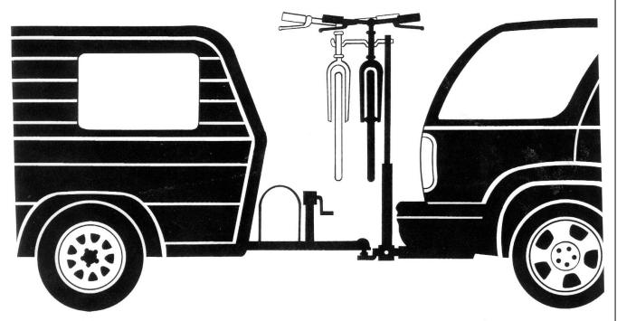
Install your trailer hitch insert tube through the base unit as far forward as possible. Tighten both set screws with hex key.
