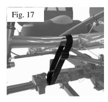
Per Fig. 17 above, the tie down straps TA-11 should be attached between the trike's frame and a tube on the bike rack. Be sure to pull the strap end through the buckle securely.
