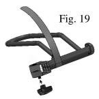
Per Fig. 19, you may need to invert the knob for the bike's front wheel holder due to limited space. Simply remove the knob and bolt and relocate the knob on the bottom.
