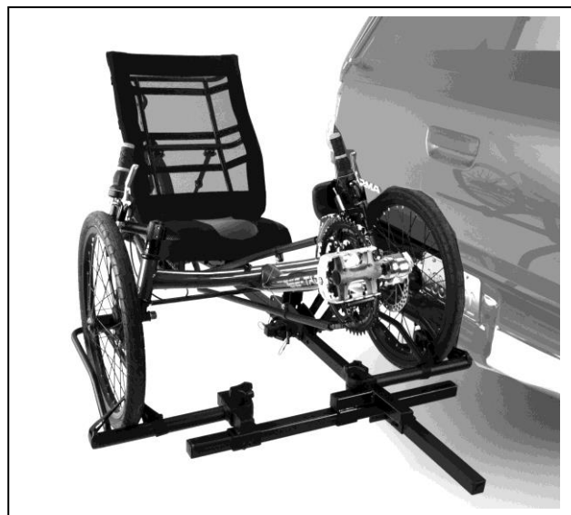
HR1000R-Y shown with mast folded down for carrying longer wheelbase tadpole
