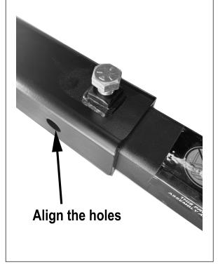
Step 2: Place the lock washer and then the flat washer onto the 1/2x13 threaded hitch pin . Insert the bolt through the hole in your receiver tube and the extender. Tighten securely with a wrench and install the R clip.
