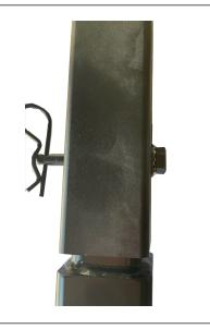
Step 4: Place the lock washer and then the flat washer onto the 1/2x13 threaded hitch pin. Insert it through the hole in the hitch extender and the rack. Tighten securely with a wrench. Next tighten the bolt on the top of the extender securely with a wrench. This will eliminate the play between the extender and the rack.
