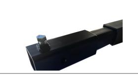
Step 3: Insert the bike racks hitch tube into the hitch extender. Align the pin holes on the rack with the holes on the hitch extender.
