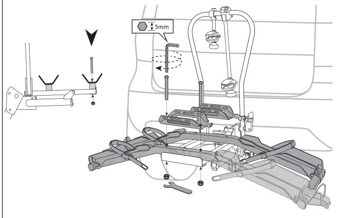
For assembly of the INSIDE bike position, the rack will need to be tilted forward. Loosen knob, tilt rack and install bridge and hardware as shown.
