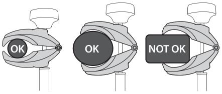
Do not attach the frame grabber to carbon frames, carbon seat posts or non-round seat posts.
