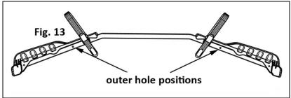
To remove strap and buckle, unscrew the knob and relocate the bolt with buckle to outer hole position. Re-install strap onto bolt and install knob. Buckle opening must be on top when inserting strap. Tighten knob securely
