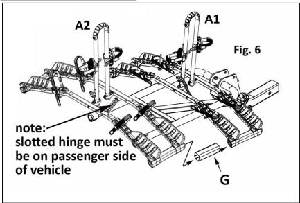
Assemble A2 to the main frame using above instructions per Fig. 5
