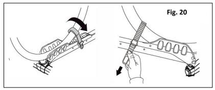
**Mounting and securing the second bike:** Fold the outer mast down.
