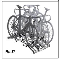
**Mounting and securing the fourth bike:** Place the bike onto the wheel trays (handlebars on passenger side). Attach the frame ratchet strap and wheel ratchet straps in the same manner as with the first, second and third bikes. See Fig. 27.
