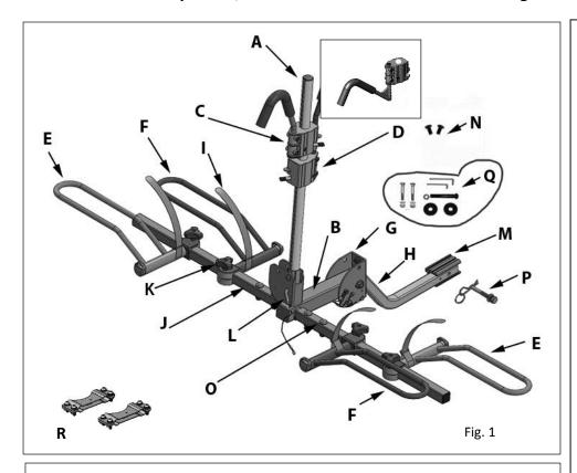
Assembly: Tools required: adjustable wrench or equivalent (3/4" or 19mm and %" or 13mm), 5 & 8mm Hex wrench included.
