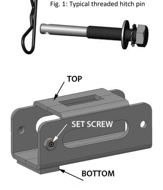
Fig. 2: Hitch Adapter
