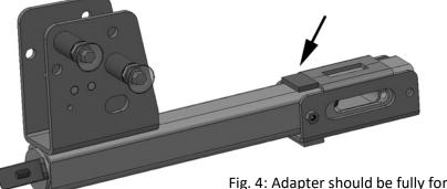
Fig. 4: Adapter should be fully forward, then tighten set screws.
