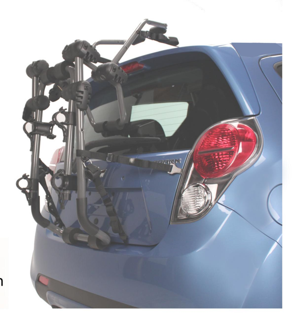
Attach upper hooks to hatch lid or trunk lid. Tighten straps by pulling on loose strap end on buckle.
