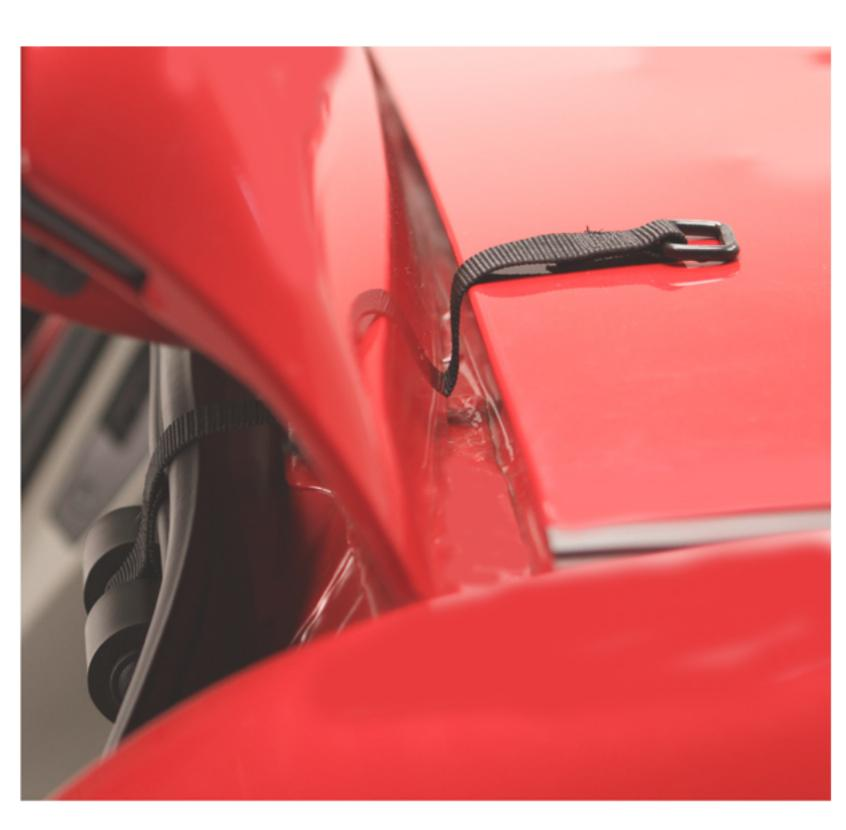
Open rear hatch and insert hatch anchor's strap with D ring through opening. Close rear hatch.
