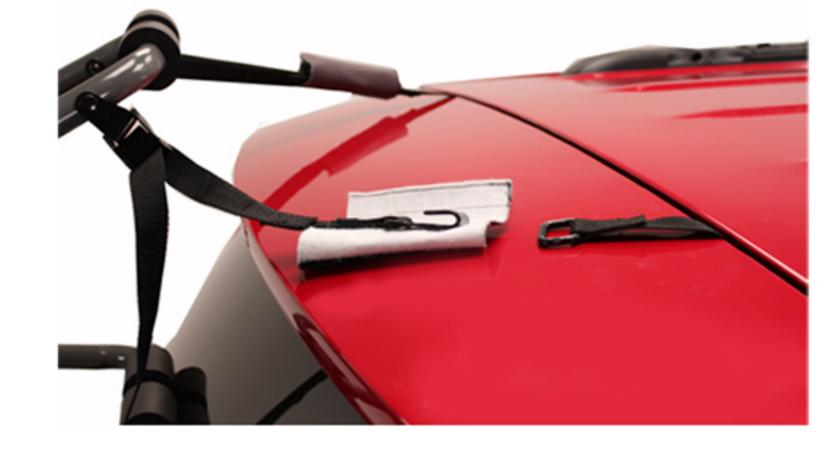
Position quick connect hook near D ring on hatch anchor.
