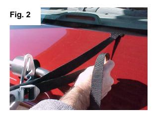
Attach the lower hooks to the bottom edge of the trunk, bumper or steel section beneath bumper and pull the end of the straps until all straps are tight. Re-tighten upper straps if necessary. Straps are shown attached to the lower edge of the trunk lid in **Fig. 3**, but they may also be attached to the bottom edge of the bumper, or loops beneath the bumper of the vehicle as appropriate to the vehicle.
