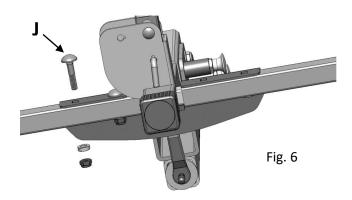
Per Fig. 6, Insert carriage bolts (J) through holes, install thick round washer and nut onto bolt end. Tighten securely with included 17mm socket tool
