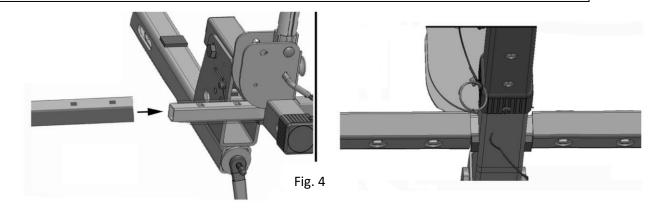
Per Fig. 4, position the wheel tubes (M) next to the square posts on the support beam (square holes on the wheel tubes should be facing up). Slide wheel tubes in so the holes are aligned.
