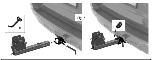
Step 1: Install Hitch Tube (B) into vehicle's trailer hitch.
