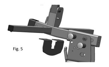
Per Fig. 5 and 6, position the brace on top of the wheel tubes. Note the brace "reaches up" from behind the wheel tubes.
