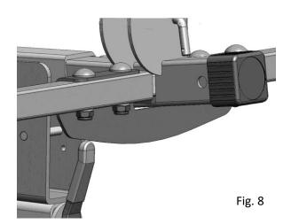
After proper assembly, wheel support tubes, brace and hardware should be per Fig. 7 and 8
