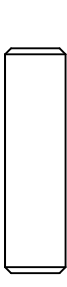
FF: M8 x 30mm Dowel x10 Goujon M8 x 30mm Pasador M8 x 30mm
