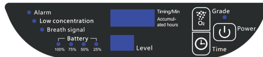
Figure 4 – Operation panel diagram
