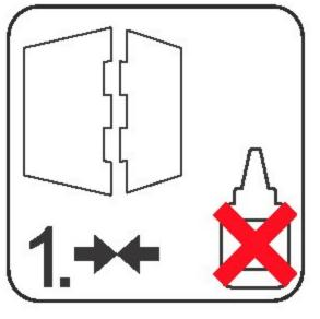
Always dry-fit the parts to together without any glue to make sure you are assembling the correct parts.
