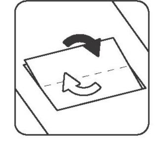
Remove the parts from the frame with a rotating motion along the axis formed by the bits you just cut.
