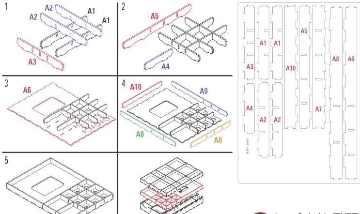
Required parts: A1x2, A2x2, A3, A4, A5, A6, A7, A8, A9, A10
