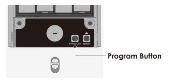
To enter **Programming Mode**, remove the battery compartment cover on the interior side of the Secure to expose the **Reset** and **Program** buttons (See page 8).
