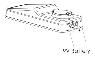
Your Lockly will automatically detect battery polarity. So hold your 9V battery lead in place against bottom of the Lockly to **temporarily** activate the screen to enter your **Access Code**. Be sure to hold the 9V battery against the contact points located at the bottom of the lock until you have successfully unlocked your door with your **Access Code**. Once unlocked, batteries should be replaced immediately.
