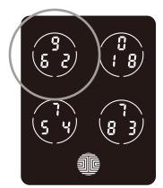
Swipe your fingers across the keypad to light up to its normal brightness. To adjust brightness, **long press the upper left button for 3 seconds.**
