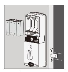
**5.1:** First install 3 of the 4 batteries. Before installing the last battery, press and hold the PROGRAM button • while installing the last battery until you hear a beep from Lockly.
