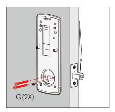
**4.3:** Without using any tools, insert 2 screws (G) on the side of the torque blade. By using hand carefully, turn the screws clockwise to catch the thread, then counter clockwise to make sure they are not cross threaded and turns smoothly. Make five turns before using a screw driver to tighten the screws until the mounting plate is securely placed to the door.
