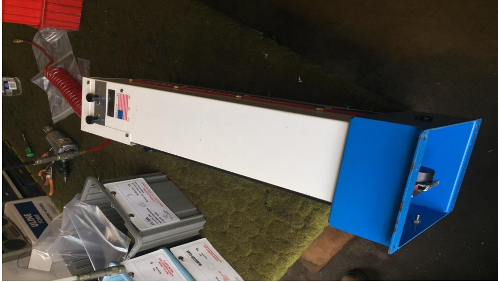
Figure 4, Lay the machine on its side with the air disconnected
