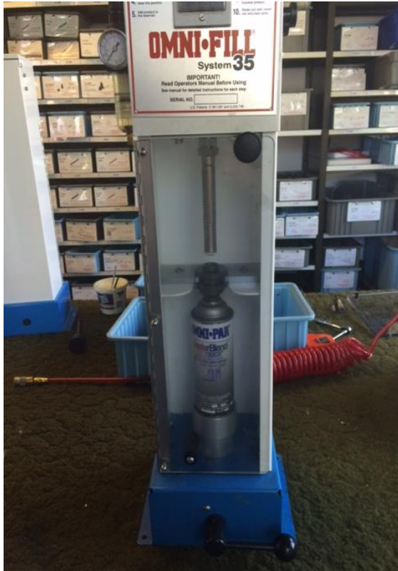
Figure 3, Insert a can and raise the platform
