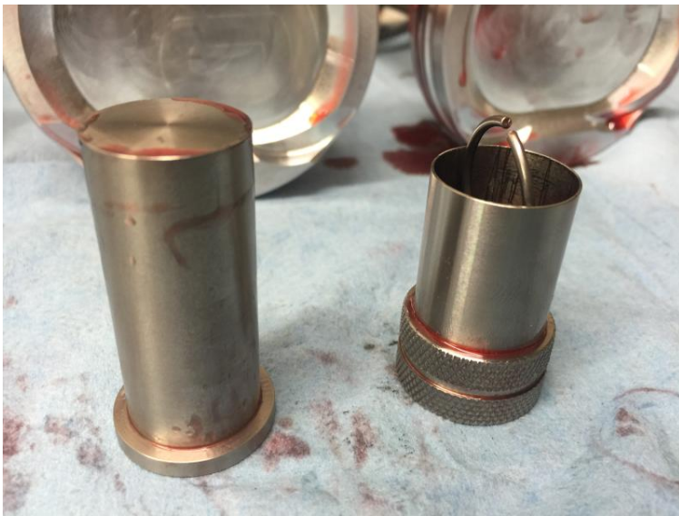
Circlip inserted into the sleeve.
