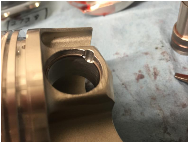
Inserted circlip. Very easy to install and no damage to the piston.
