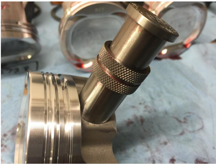
Pressing the circlip into the piston.
