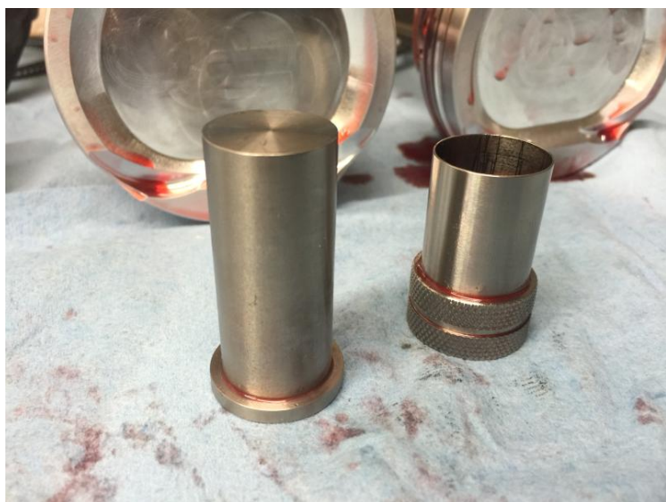
Male and female parts of the Circlip Injector(TM).
