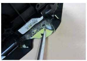
Cut the cover at the corners of the button recess to allow it to fold in easily. Do not cut all the way to the edge or the cut will be visible once folded.
