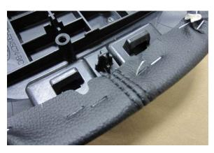
Remove the staples around the perimeter with a small flat head screwdriver. You may need pliers to completely remove them. Once all of the staples are out, you can remove the factory cover.
