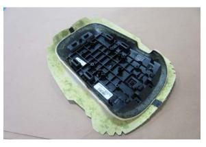
If you are not using a staple gun for attachment of your new cover, apply adhesive to only the outer portion of your new cover and only the inside edge of the console lid. Allow the adhesive to become tacky. Align the seam lines so that they correspond with the small indentions on the center of the front and rear edge of the console lid.
