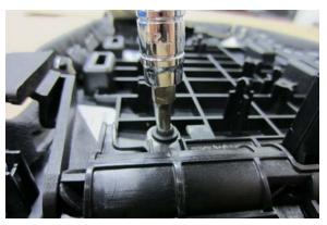
Remove the release levers by unscrewing the two T20 hex screws from the base of the console lid.
