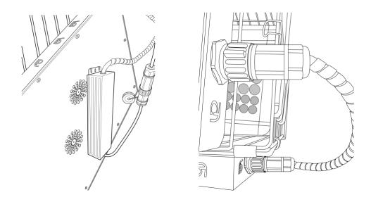
8. The ON/OFF switch is found on the back panel, right side. Red is for the red bulbs and green is for the Near-infrared bulbs (when on, the bulbs will show a very dull red light).
