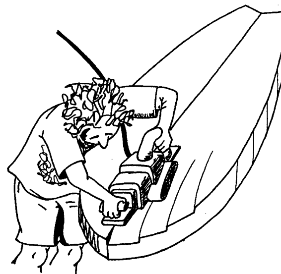
FIG. 6-9 SHAPING NOSE FOR ROCKER
