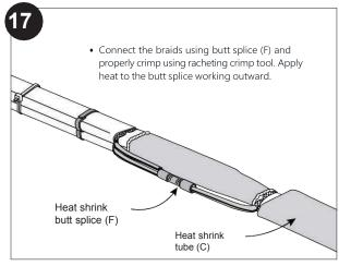
• Slide shrink tube (C) over splice as shown.
