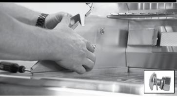
Using your 10mm wrench and phillips screwdriver hold screw and tighten the nut.
