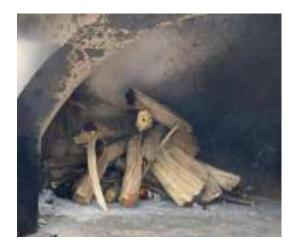
Use the wax ignition block in order to ignite the firewood. The size of the ignition firewood is about 20 x 30 x 200mm. After the firewood is completely burned for 3 minutes, move to the air outlet hood of the furnace. Then, add new wood, start the combustion supporting fan, and adjust the fan controller to medium speed (indicator light should be green).
