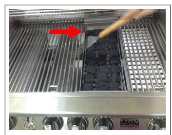
**Step 4:** Use spatula to move the grate to cooking area or push aside charcoal. Please move the grate on top of the charcoal tray before ignition to pre-heat the grate.
