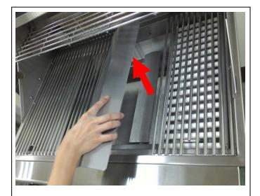
**Step 1:** Remove grate and flame tamer or ceramic tubes with flat tray first.
