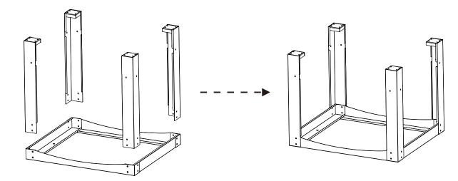
STEP 3 - Attach 2 x side shelf (7) to STEP 2 as shown on below diagram. Fix them using 16 x M8\*20 bolts (A),16 x Φ8 washers (B) and 16 x M8 nuts(D).
