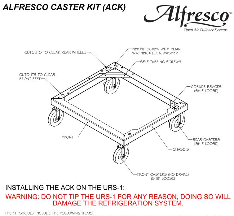
CHASSIS (1), CORNER BRACES (4), CASTERS (2 WITH BRAKE ¢ 2 WITHOUT BRAKE), 8-32 X 1/2 SELF TAPPING SCREWS (8), 1/4-20 X 1/2 HEX HD MACHINE SCREWS (4), 1/4 FLAT WASHERS (4) 1/4 HELICAL SPRING LOCK WASHERS (4) AND THIS INSTRUCTION SHEET.
