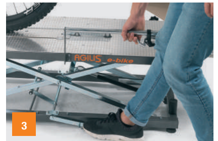
3 Press the safety pedal and effortlessly lift Agilis® to the desired height
