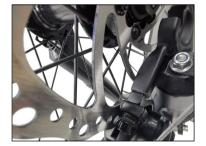
Step 5: Prepare your quick-release skewer for the next step by removing the thumb nut and one of the cone springs.
