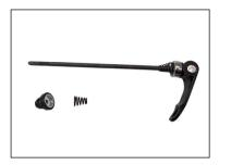
Step 6: Install the quick-release skewer starting from the brake rotor side of the wheel. Inserting the quick-release skewer through and then install the second cone spring on the other side. Ensure the narrow side of both springs towards the wheel hub.
