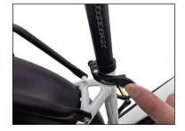
**Warning:** Overextending the seat post can cause it to break or come off your bike, which will put you at very high risk of serious injury or death. Avoid this danger by inserting your seat post into the seat tube far enough that the minimum insertion point is no longer visible. !
