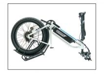
Step 2: Remove the plastic axle guards from the front wheel being careful to avoid contacting the brake rotor set.
