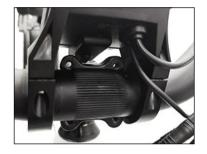
Step 3: Tighten bolts to handlebar stem, but don't tighten completely as you may want to further adjust the angle later to align more precisely. Test the position and adjust the handle bar to your favorite angle. After determining the best position, completely tighten all the bolts on the stem.
