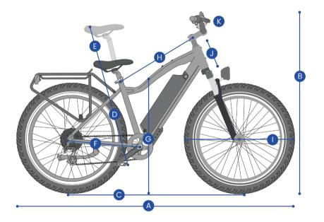
A -- Total Length 75" B --- Handlebar Height 46.5" C --- Wheelbase 45" D --- Minimum Seat Height 28" E -- Maximum Seat Height 36.5" F --- Chain Stay Length 19" G --- Standover Height 31" H --- Top Tube Length 22.5" I -- Wheel Diameter 28" J -- Head Tube Length 6"
