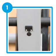
Locate the sensor under the slideway
