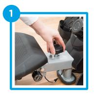
Start by unscrewing the knob closest to the base of the machine
