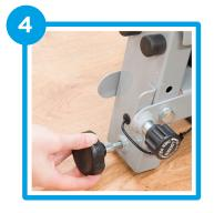
Reattach the knob on the underside of the slideway
