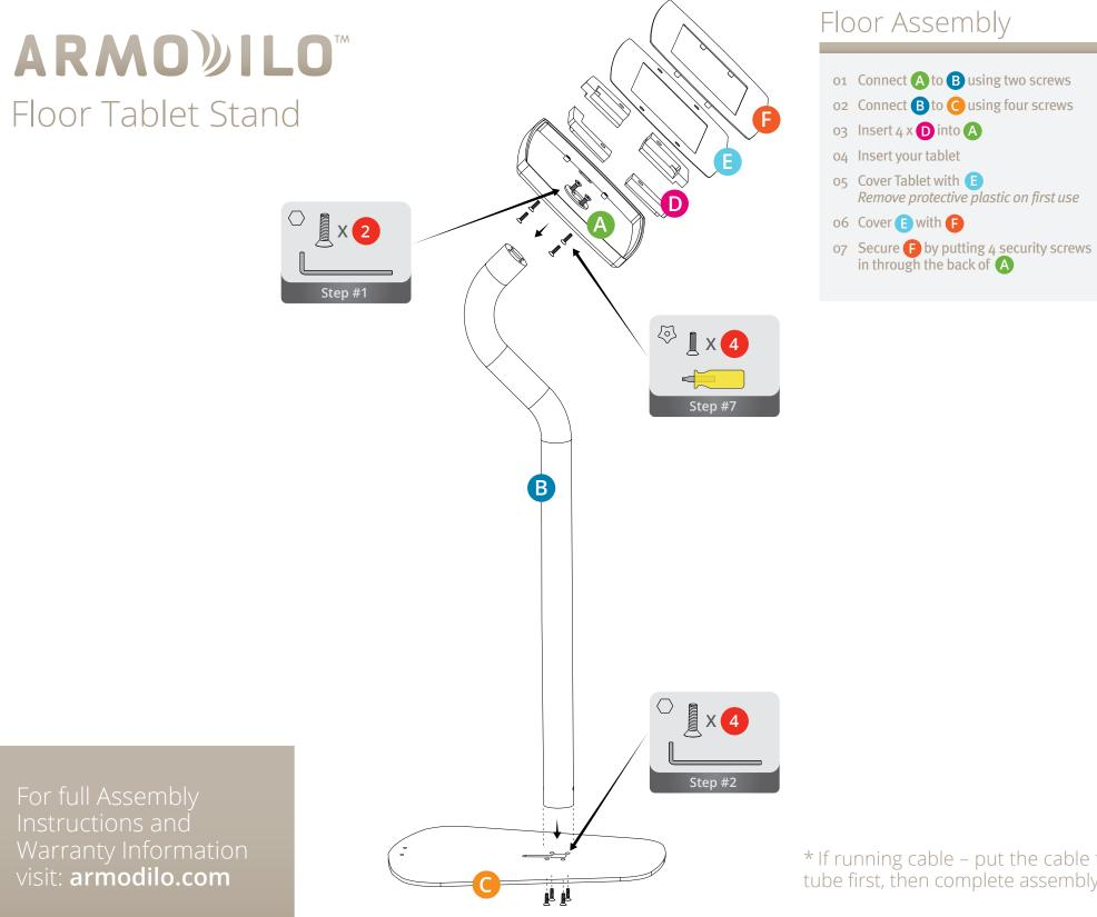
\* If running cable – put the cable through tube first, then complete assembly as noted
