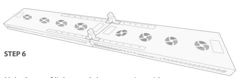
Make 2 sets of light panels by connecting with light bracket pieces. Prepare to slide each set onto the stand arm.
