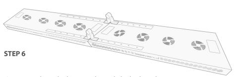
Connect the 2 light panels with light bracket extensions and bracket pieces using 20x light breacket bolts. Prepare to slide the set as one onto the stand arm.
