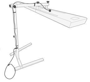
Insert the bracket loops onto the arm, install in first or second hole with knobs. Install & Secure the cord using the Velcro straps.
