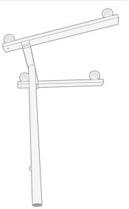
Set Stand upright and lock all wheels. Install the neck with the longest thumb knob, then install the arm.
