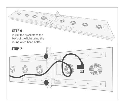
Insert the bracket loops onto the arm, install in first or second hole with knobs. Install & Secure the cord using the Velcro straps.
