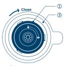
Secure the ① cap by turning it clockwise.
