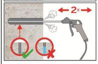
Finally blow the bore hole clean minimum 2x with compressed air (min. 6 bar, oil-free) (Annex B 4) over the entire embedment depth until return air stream is free of noticeable dust. (If necessary, an extension shall be used.)
