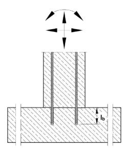
Figure A2: Slab / beam to wall or beam to column
