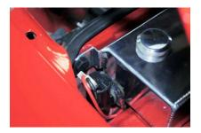
10. Mount the included rubber grommet to the firewall hole near the OE connector on the passenger side and route wiring along the firewall with supplied clips so that the wire loom is kept away from the wiper arm mechanism. \*ABS-equipped models will need to route this along the driver's side fender.\*
