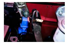
11. Pass the wire loom through the rubber grommet, strip the ends, and crimp the male electrical blade connectors to the two wires.
