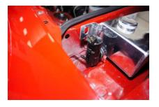
6. Mount rubber pad on bottom of tank as indicated.
