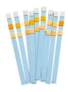
Designed specifically for hydrogen water, these strips are essential for assessing water before and after hydrogenation. A low quality water source can damage the Proton Exchange Membrane (PEM) in your Hydrogen Water Generator.
