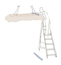
4.ONCE THE INSTALLATION IS COMPLETE, REMOVE THE TWO BATTENS BY RELEASING THE CABLE TIES.
