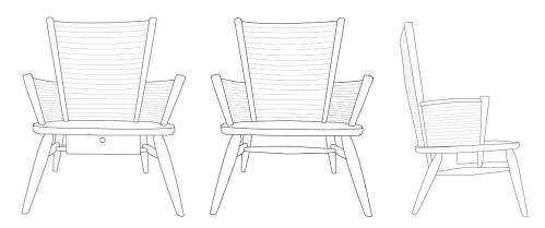
H880X W720 X D550mm, W12.5kg SEAT HEIGHT 330 mm
