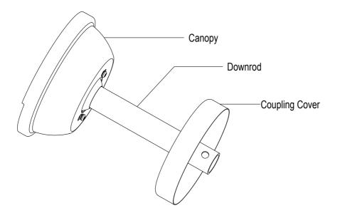
**Step 2** - Route the all the wires from the motor through the downrod. Fix the downrod to the coupling with bolt, washer, nut and tighten them firmly then insert the clevis pin.
