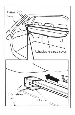
3: While pulling back on the plastic cap, Insert the left side holder of the retractable cargo cover into the trunk side trim installation receptacle.
