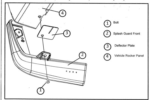
5. Loosely install (2) kit bolts. Use care to ensure bolts are not cross-threaded as damage could occur. Note the area where the double sided tape square on the deflector plate contacts the body panel.
