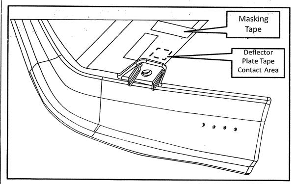
9. Remove pull-rivet, remove flag from the double-sided tape, and press part securely to vehicle.
