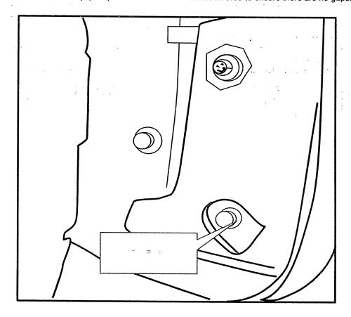
7. Mark the deflector plate location with pieces of masking tape. Remove bottom bolt and slide out deflector plate.
