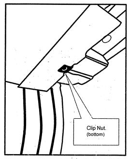
4. Loosely install deflector plate, splash guard, and bolt in the order shown below. There are LH and RH deflector plates. Install on the correct side with the tape side facing up. Deflector plate has a scribe line that should approximately line up with the edge of the vehicle rocker panel. If it does not line up, make sure they are installed on the correct side. Note: At this time do not peel tape backing off deflector plate. This is a dry fit only.
