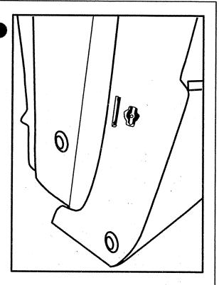
2. Cut out existing top, hour glass plastic tab using a nipper. Then cut the larger plastic tab next to it to create a shallow rectangular slot. Remove lower pull rivet.
