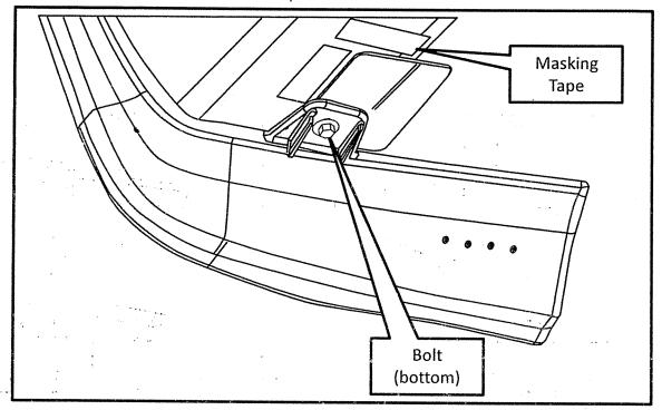
8. Clean the area where the double sided tape square on the deflector plate contacts the body panel with alcohol wipe. Let area dry then apply adhesive promoter. Allow adhesive promoter dry for 30 seconds. Slide the deflector plate back into correct position and loosely install bottom bolt. Make sure the bolt threads into the clip nut. Remove tape backing on deflector plate and press deflector plate firmly onto the rocker panel to adhere the double sided tape. Remove masking tape.
