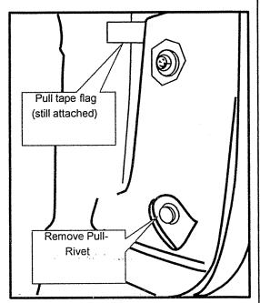
11. Re-install pull-rivet and torque bolts in order shown in the figure on the left while pressing the splash guard against the over fender.
